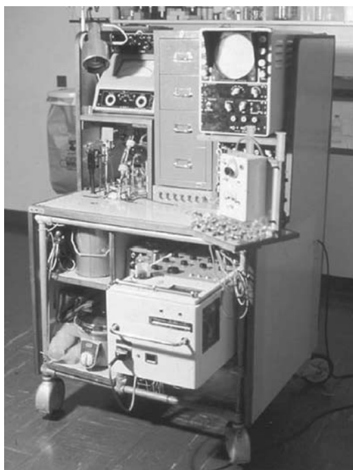
Fig. 3-12. Portable equipment used to study cardiac function, designed by Bradley and colleagues
